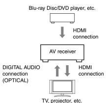
Connect the audio output from the TV to the OPTICAL IN 2 jack of the AV receiver using an optical digital cable.
